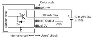
Note: The output does not incorporate a short-circuit protection circuit. Do not connect it directly to a power supply or a capacitive load.
