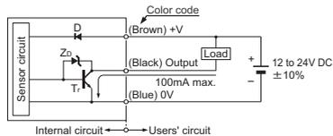
Symbols: D: Reverse supply polarity protection diode
