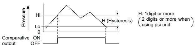
Note: "Hi-1" or "Lo-1" is displayed for comparative output 1 and "Hi-2" or "Lo-2" for comparative output 2 on the sub-display.
