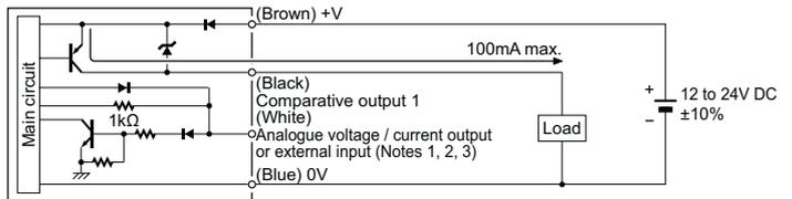
Notes: 1) When the analogue current is output, the output load resistance should be 250Ω max.
